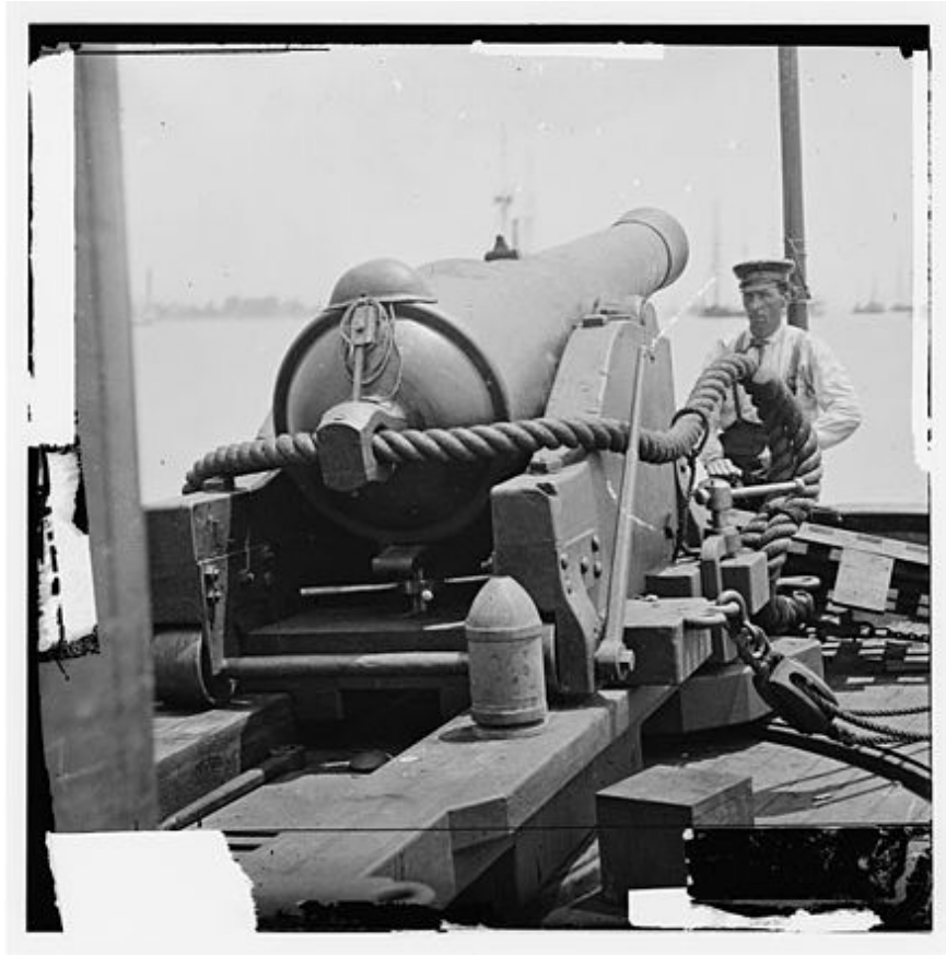
6.4-inch banded rifle, the weapon type used as the bow pivot gun on the CSS Ivy. Note the 100-pound conical projectile at the right rear of the gun carriage
